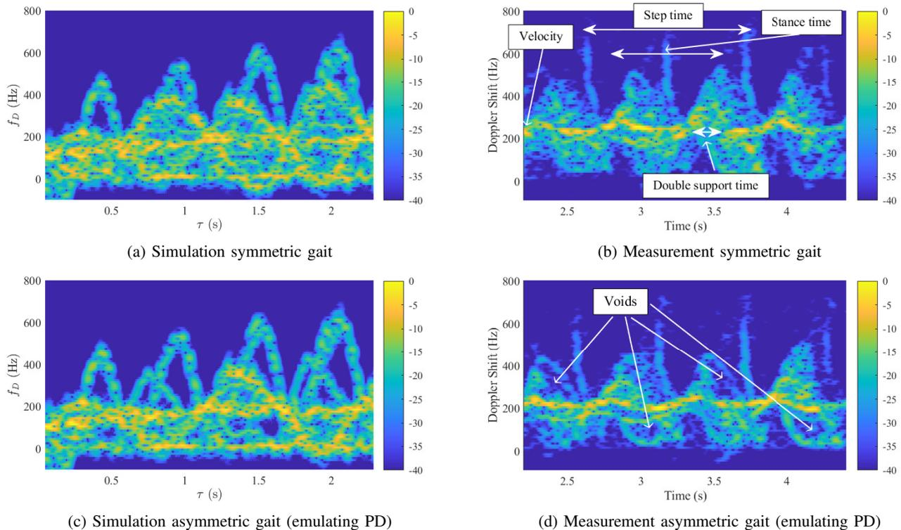
Fig. 6: Micro-Doppler signatures of (a) and (b) a person with symmetric gait (healthy), (c) and (d) a person with asymmetric gait, emulating PD. (a) and (c) are simulations carried out using the techniques presented in [18], using the recording of subject 2 of [19]. (b) and (d) are measurements carried out with the radar node designed placed 1.2 m above the ground using the configuration shown in Table I.
