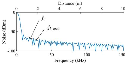
Fig. 4: Noise of the system using the radar MMIC Silicon Radar TRX-024-046 with an FFT bandwidth  $B_{\text{FFT}} = 1.2$  kHz, and  $N_{\text{FFT}} = 256$  bins. It is selected  $f_{b \min} = 30\text{kHz} \geq f_c$ . In the top axis it is represented the distance to the target considering  $B = 1.4$  GHz, and  $T_c = 625\mu\text{s}$ .
