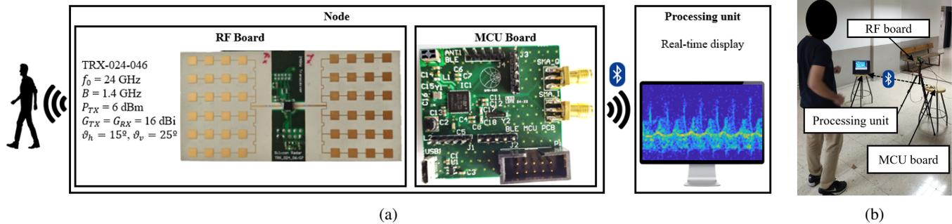
Fig. 5: (a) Node and processing unit schematics, with the different boards of the node: RF board with the MMIC and antennas, and MCU board for signal conditioning and acquisition. (b) Real-life measurement: the MCU board samples the IF signals, and transmits them to a processing unit via Bluetooth.
