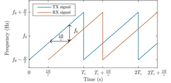
Fig. 3: Working principle of LFM-CW radar. The range of the target  $R$  is proportional to the beat frequency  $f_b$ : the frequency difference between the transmitted and received signals.
