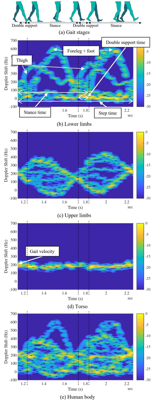
Fig. 1: Simulation of the micro-Doppler signature of the different gait stages (represented in a) focusing on: (b) lower limbs, (c) upper limbs, (d) torso, and (e) complete human body. Some metrics are included in the signatures. It is used the recording of subject 2 of [19]. The radar simulated is a 24-GHz LFM-CW radar with chirp time  $T_c = 625\mu\text{s}$ , and bandwidth  $B = 1.4$  GHz.
