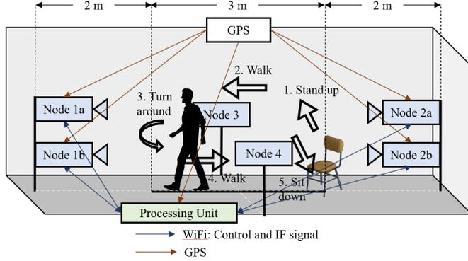
Fig. 2: Measurement environment with a target performing the TUG test. The system must work in small rooms such as the ones in a hospital. All nodes must capture a 1.8 m tall person 2 m away from the node. Nodes 1b and 2b are 0.4 m above the ground, and nodes 1a, 2a, 3, and 4 are 1.2 m above the ground.
